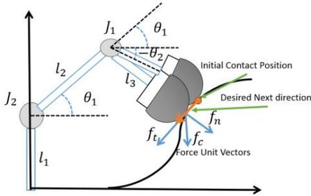
Figure 1 Force control diagram with 2DOF finger
