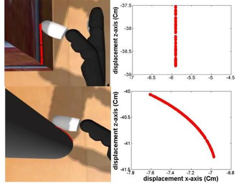
Figure 7 The trajectory result of surface following with position control As shown in figure 7, the controller performs well when following the straight and the curved geometries.
