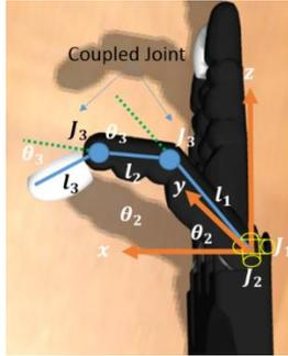
Figure 5 Shadow hand finger(3DOF) diagram
