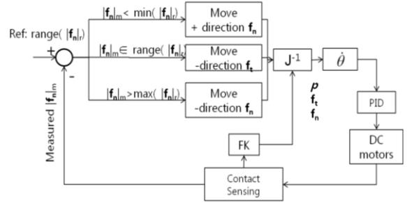
Figure 2 surface following control system with velocity control
